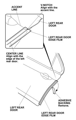
19. Align the center line on the left rear door edge film with the edge of the left rear door. While applying light pressure, carefully remove the adhesive backing.
