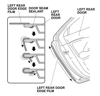
23. Using a shop towel, wipe the excess 3M protective tape application solution from the left rear door edge film. Allow the left rear door edge film to dry thoroughly.
