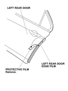
22. Starting from the center and working outward, use your finger and the applicator to fold the left rear door edge film inside the left rear door as shown.
