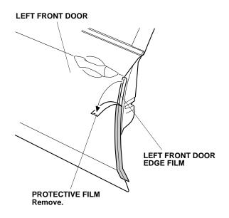
11. Starting from the center and working outward, use your finger and the applicator to fold the left front door edge film inside the left front door as shown.
